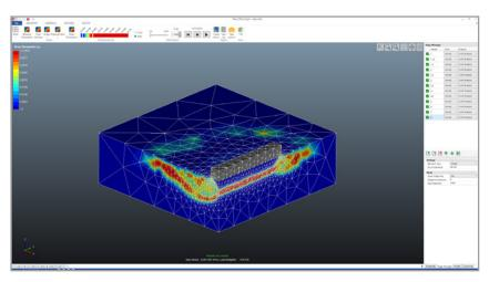
Automatic adaptive mesh refinement ensuring maximum accuracy at minimum computational cost.
